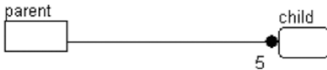
Figure 3-5. One-to-exactly N (in this case, 5, meaning each parent must have five children)
