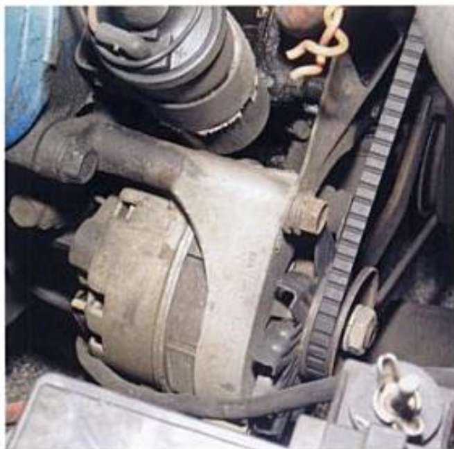
Fig 5-9. A charge light indicator receives power from the ignition switch and ground from the voltage regulator. When the alternator starts turning, the ground for the voltage regulator's light builds voltage until the indicator light eventually has no ground and goes out.
