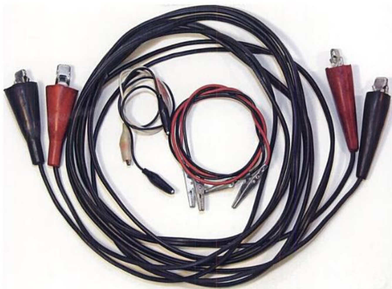
A personal can never have too many jumper wires. They come in all different sizes, as shown here. The large set of jumpers was homemade using 14-gauge lamp cord; it comes in mighty handy for getting power from the front to the back of a vehicle or trailer.
