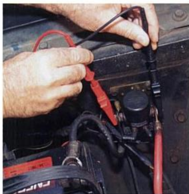
This remote starter solenoid can easily be checked for high resistance using a voltage drop test. The contacts inside the solenoid should not exceed a drop of 0.2 volt during starter cranking.
