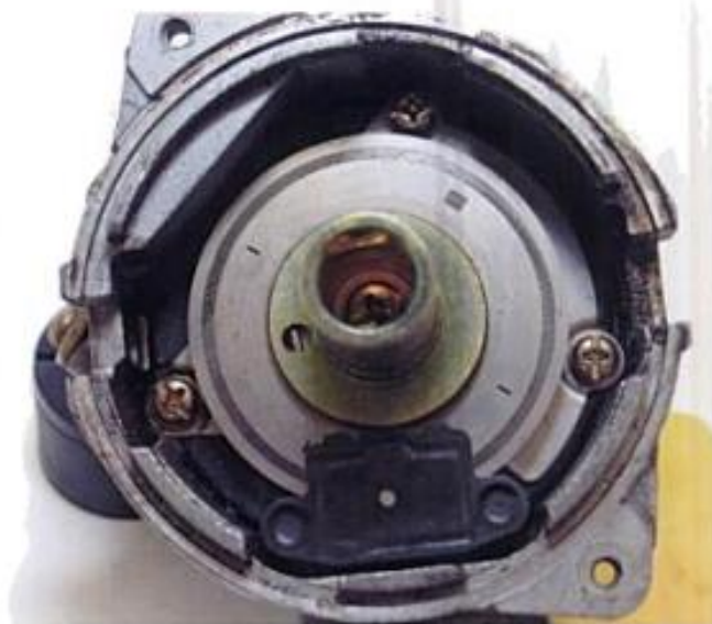
Inside this optical distributor there are 360 holes on the outer ring of the metal disk—one for each crankshaft degree. The inner ring has four holes, one for each cylinder. The large hole is for cylinder number one in the engine's firing order.
