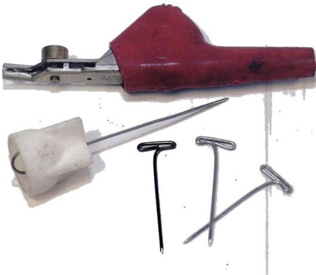
A JS Popper alligator clip (top) equipped with a bed-of-nails. This tool can pierce wire insulation and provide a place to connect a voltmeter. The T-shaped pins (bottom) are available from any fabric store and work well to back probe connectors.
