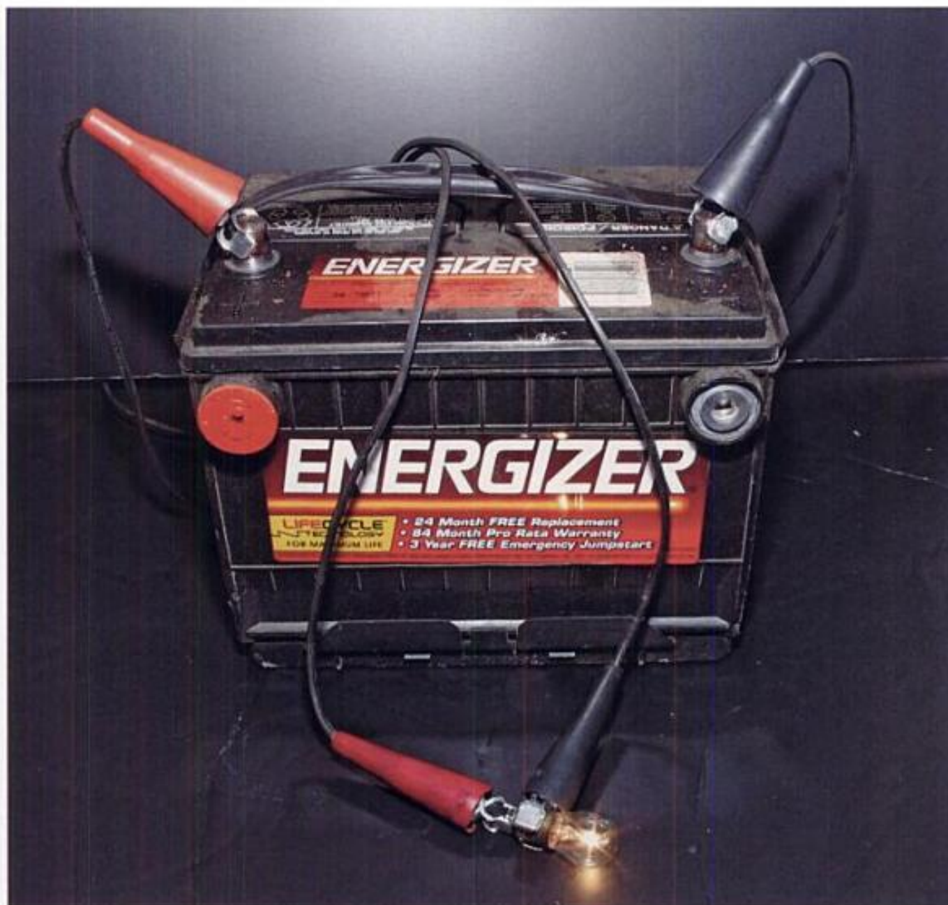
A simple 12-volt battery, wires, and light bulb make up a basic DC circuit.
