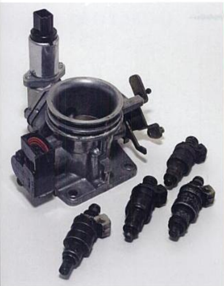
This Ford throttle body and injectors make up a modern EFI system, providing better performance and fuel mileage than the carburetors of the past.
