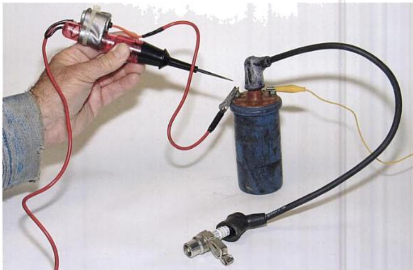
This ignition coil is being bench-tested. The yellow wire is 12 volts and the wire coming out of the coil tester goes to ground. When the pointy end of the coil tester is tapped on the negative coil terminal, a spark is produced.
