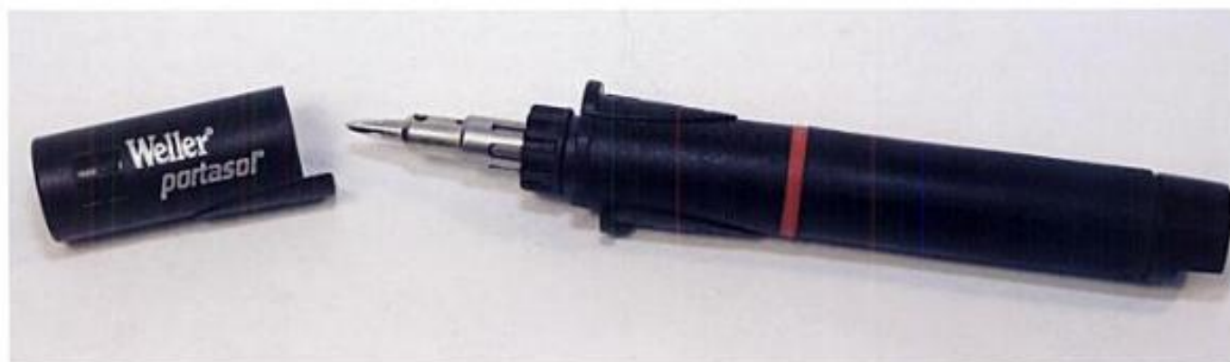
Weller's Portasol—a completely portable, butane-powered soldering iron. This tool is convenient and invaluable when working on trailer wiring, under the dash, at the racetrack, or on those dreaded roadside repairs. Heat is adjustable and ignition is via a piezoelectric system—just flick the ON switch. The tool can be charged with butane using the same canisters that fill cigarette lighters. One fill-up lasts several hours—more than enough time to solder entire wiring harnesses. Courtesy of Weller
