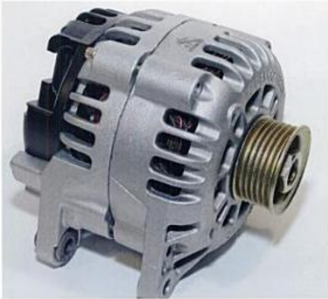
GM produces two CS alternators that can be identified by the letters on the plastic plugs at the backs of the cases. Each plug will read either PLIS or PLFS. These alternators are not interchangeable, so make sure the correct one for the vehicle is installed. Courtesy CARQUEST Auto Parts
