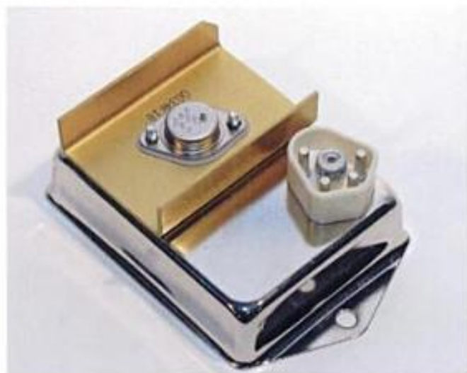
This Chrysler ignition module uses a large transistor mounted in a gold-colored aluminum heat sink (upper left of module). Courtesy of CARQUEST Auto Parts
