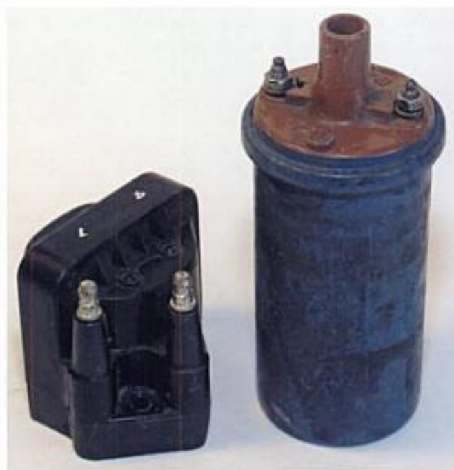
The difference between the DIS coil (left) and a conventional coil is that the DIS coil's secondary windings are not connected to the primary circuit. This design causes the spark produced by a DIS coil to go to the other side of the secondary windings and not the battery ground.
