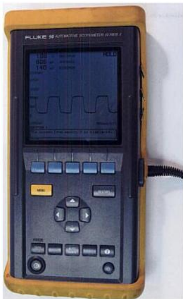
A Fluke 98 Scope Meter can record and play back both analog and digital electronic fuel-injection signals. It can also measure secondary ignition voltage and display spark plug firing patterns. Courtesy of Fluke Corporation
