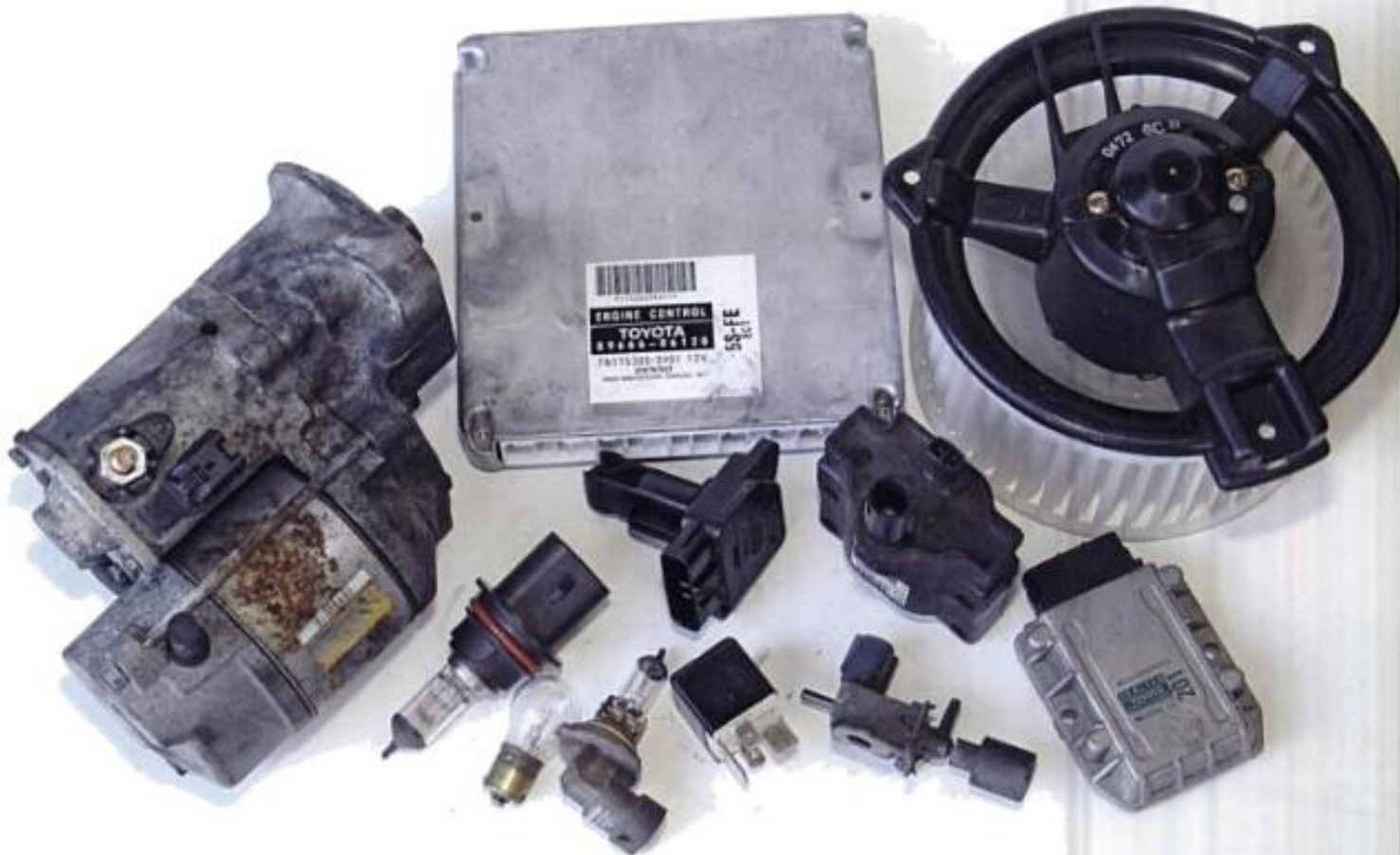
These components may appear different, but they're all just load devices with resistance to electron flow. Courtesy Younger Toyota
