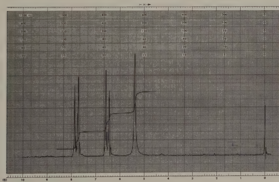
Spectre 31.2 Spectre de RMN de la nitro-4 aniline (solution dans \text{CDCl}_3 , \text{DMSO-}6\text{D} , 3/2)
