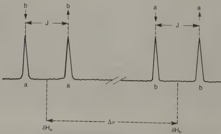
Figure 23.10 Couplage vicinal ^3J_{\text{H}_a-\text{H}_b} ( \delta\text{H}_a - \delta\text{H}_b \gg |^3J| )
