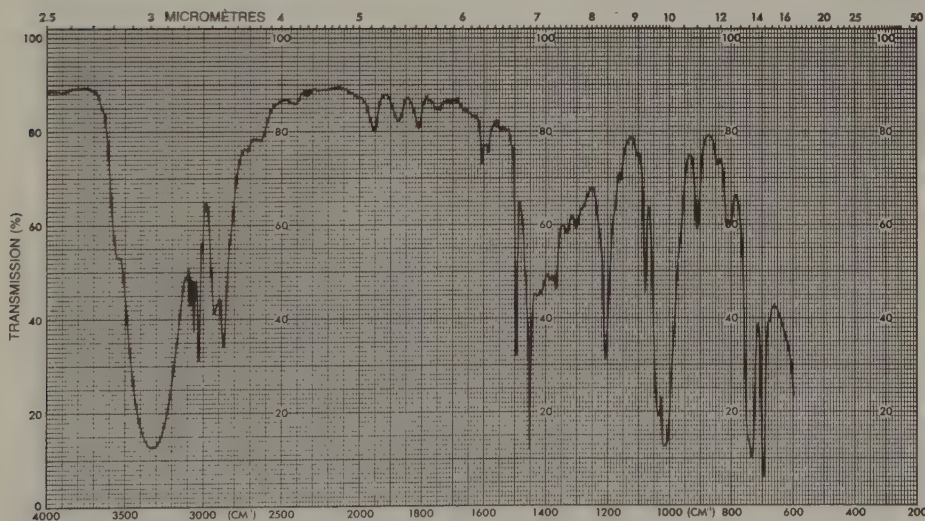
Spectre 37.1 Spectre IR de l'alcool benzylique (liquide pur en film)
