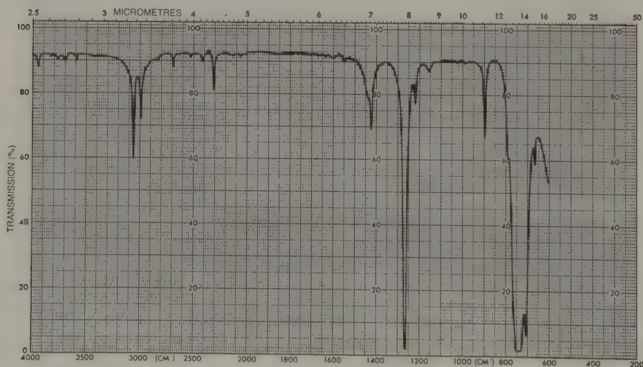
Spectre 22.2 Spectre IR du dichlorométhane (liquide pur en film)
