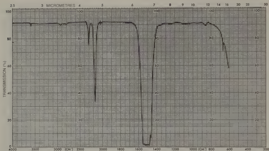
Spectre 22.5 Spectre IR du sulfure de carbone (liquide pur en film)
