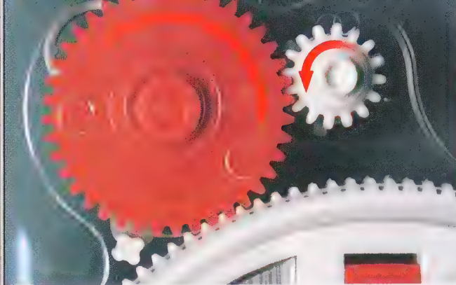
Figure 20 If an input force is applied to the larger gear and it rotates clockwise, the smaller gear rotates counterclockwise. The output force exerted by the smaller gear is less than the input force applied to the larger gear.
