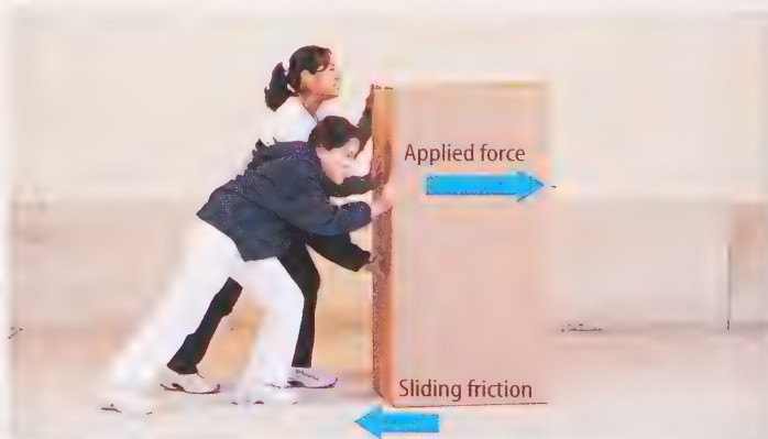
Figure 15 Sliding friction acts on the sliding box in the direction opposite to the motion of the box.
