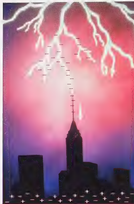
Figure 9 A lightning rod directs the charge from a lightning bolt safely to the ground.
