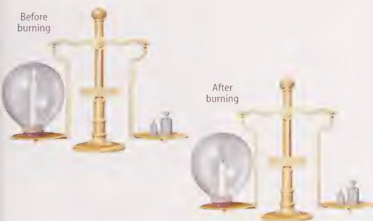
Figure 2 The mass of the candles and oxygen before burning is exactly equal to the mass of the remaining candle and gaseous products.
