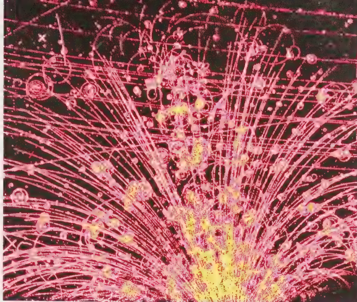
Figure 12 Particles of nuclear radiation can be detected as they leave trails of bubbles in a bubble chamber.
