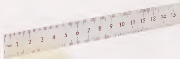
Figure 11 This metric ruler has centimeter and millimeter divisions.
