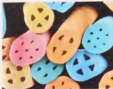
Figure 17 The fibers of this insulating material contain air spaces that are good thermal insulators. They reduce the rate at which thermal energy flows in the material.
