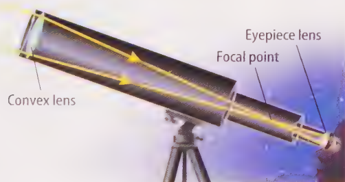
Figure 2 Two lenses are all that is needed for a refracting telescope. The tube and tripod aid in viewing.
