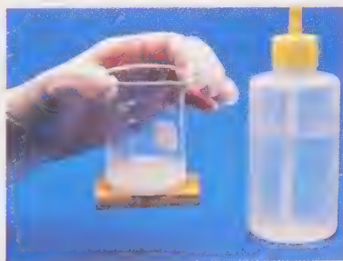
Figure 17 As an endothermic reaction happens, such as the reaction of barium hydroxide and ammonium chloride, energy from the surrounding environment is absorbed, causing a cooling effect. Here, the reaction absorbs so much heat that a drop of water freezes and the beaker holding the reaction sticks to the wood.
