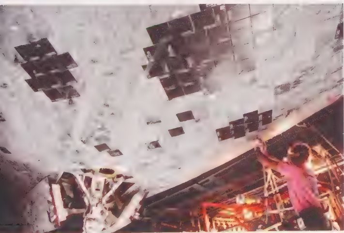
Figure 4 NASA has had an ongoing mission to improve the space shuttle. A technician is replacing tiles damaged upon re-entry into Earth's atmosphere.
