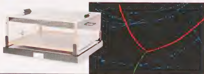
Figure 11 If a sample of radioactive material is placed in a cloud chamber, a trail of condensed vapor will form along the paths of the emitted particles.
