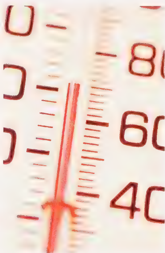
Figure 11 The liquid in the thermometer tube expands as its temperature increases. Because the tube expands much less than the liquid, the height of the liquid column increases as the temperature increases.
