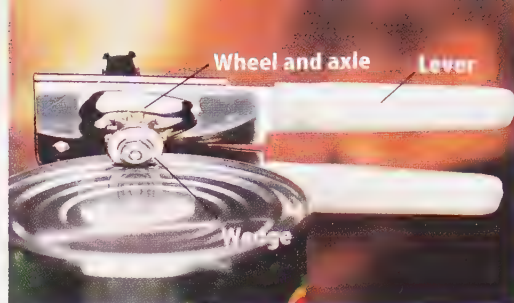
Figure 23 A compound machine, such as a can opener, is made up of simple machines.
