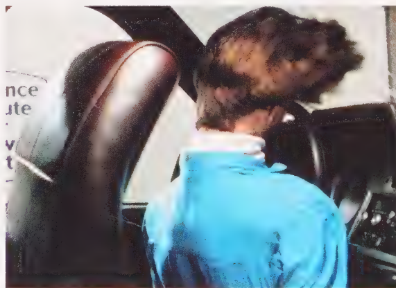
Figure 4 This crash test dummy is not restrained in this low-speed crash. Inertia causes the dummy to slam into the steering wheel.
