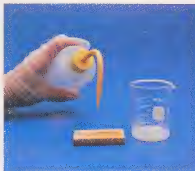
Figure 17 As an endothermic reaction happens, such as the reaction of barium hydroxide and ammonium chloride, energy from the surrounding environment is absorbed, causing a cooling effect. Here, the reaction absorbs so much heat that a drop of water freezes and the beaker holding the reaction sticks to the wood.
