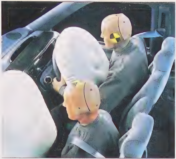
Figure 5 These crash test dummies were restrained with safety belts in this crash. This prevented the dummies from hitting the dashboard or windshield.
