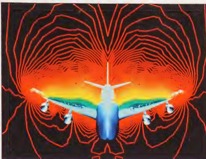
Figure 15 This is a computer simulation of an aircraft in a wind tunnel. The lines and colors surrounding the aircraft show airflow and turbulence. Scientists who use computer simulation can work to improve the aircraft design.
