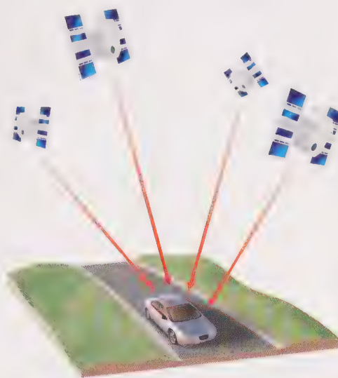
Figure 22 A GPS receiver uses signals from orbiting satellites to determine the receiver's location.
