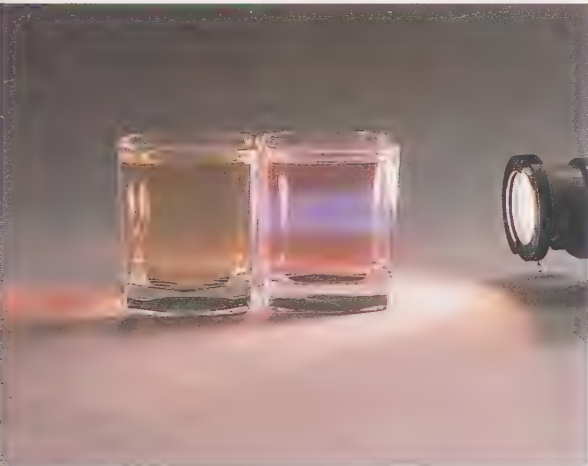
Figure 8 Because of the Tyndall effect, a light beam is scattered by the colloid suspension on the right, but it passes invisibly through the solution on the left.
