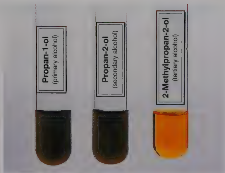
• Figure 11.5 The colour changes that occur when primary, secondary and tertiary alcohols are treated with hot, acidified potassium dichromate(VI).
