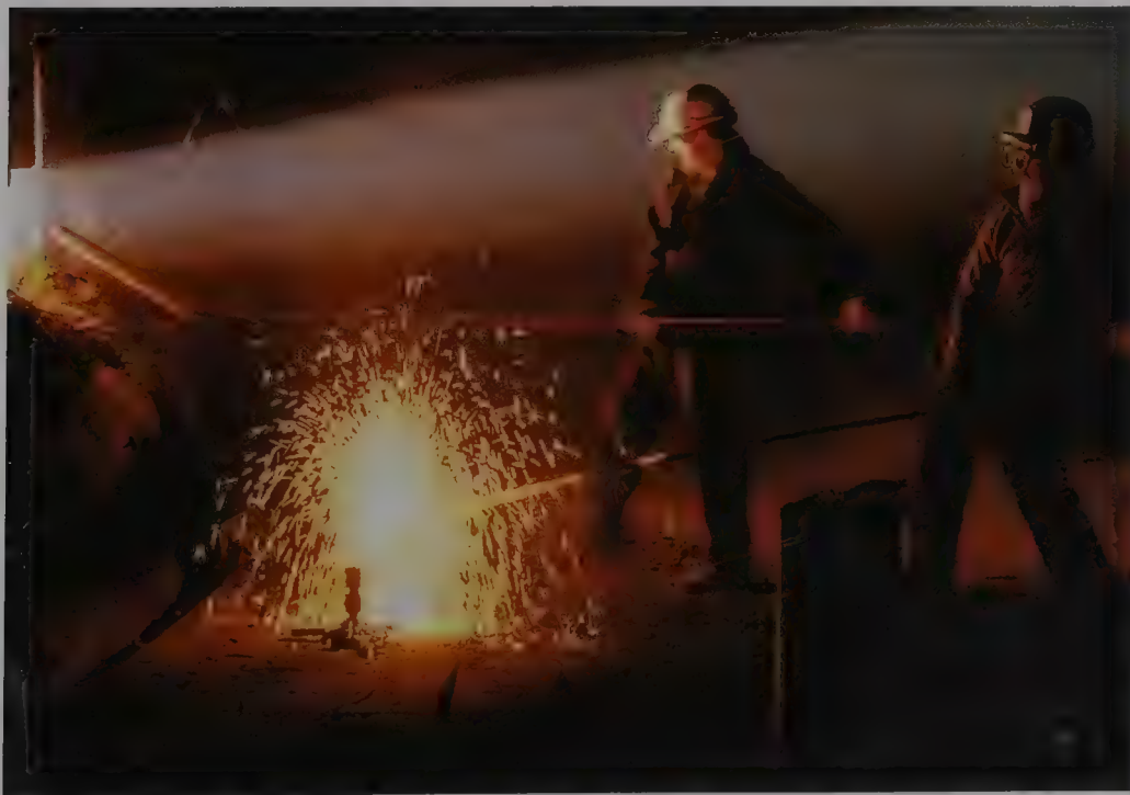
● Figure 2.6 Workers taking the slag from the top of the molten iron in an open-hearth blast furnace.
