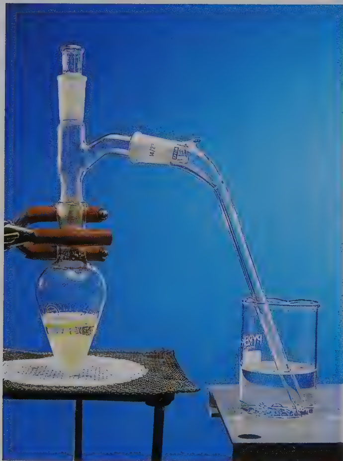
● Figure 11.4 Bromoethane forms when a mixture of ethanol, concentrated sulphuric acid and sodium bromide crystals is heated. The product distils from the reaction mixture and collects as oily droplets under water.
