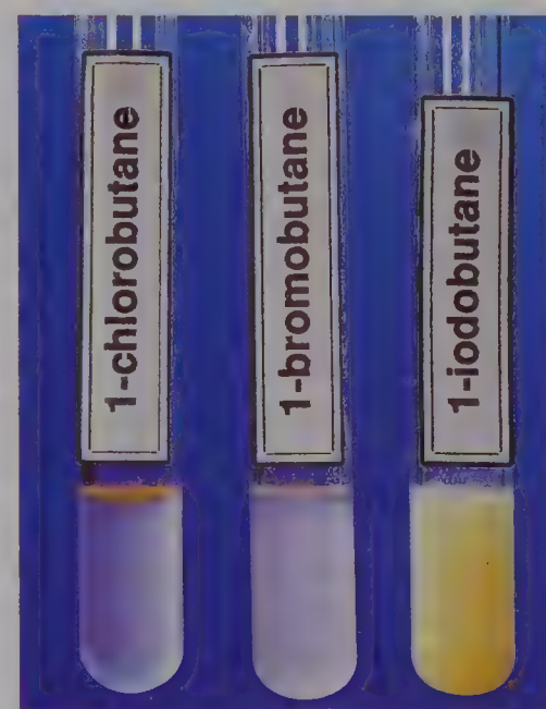
● Figure 12.2 The hydrolysis of halogenoalkanes by aqueous ethanolic silver nitrate after 15 minutes. The silver nitrate produces an insoluble precipitate of a silver halide.
