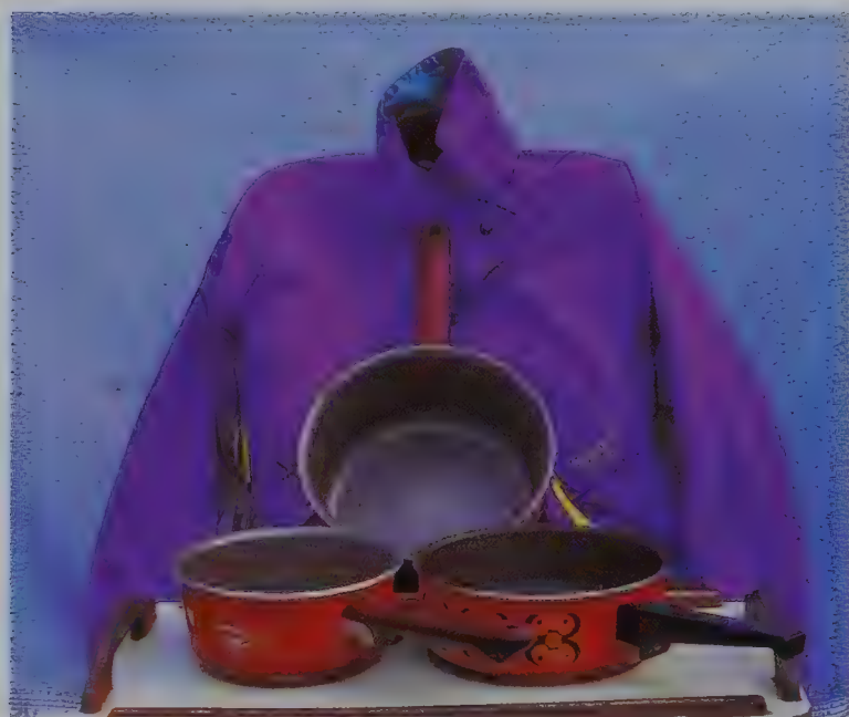
● Figure 12.3 Poly(tetrafluoroethene), PTFE, is used in the non-stick coating on saucepans and in waterproof clothing.
