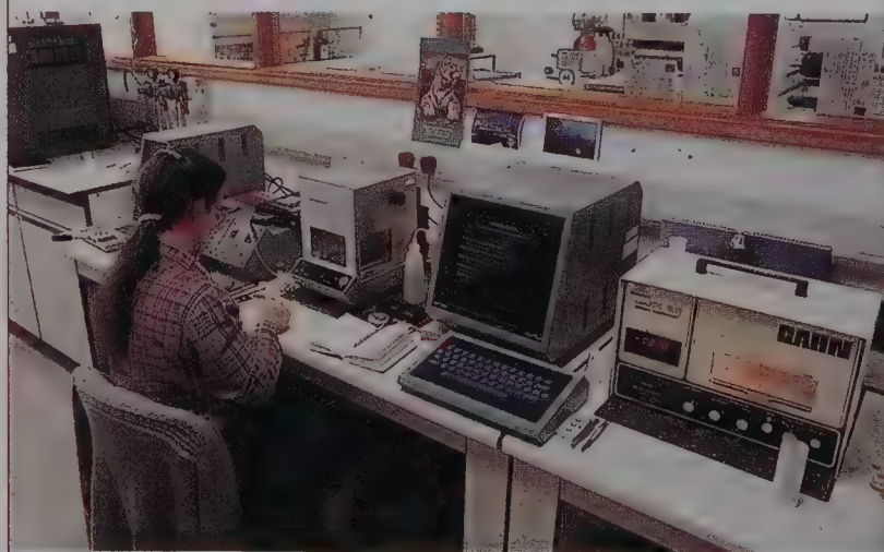
● Figure 2.7 Modern microanalytical equipment used for routine determination of percentage of carbon and hydrogen in a compound.
