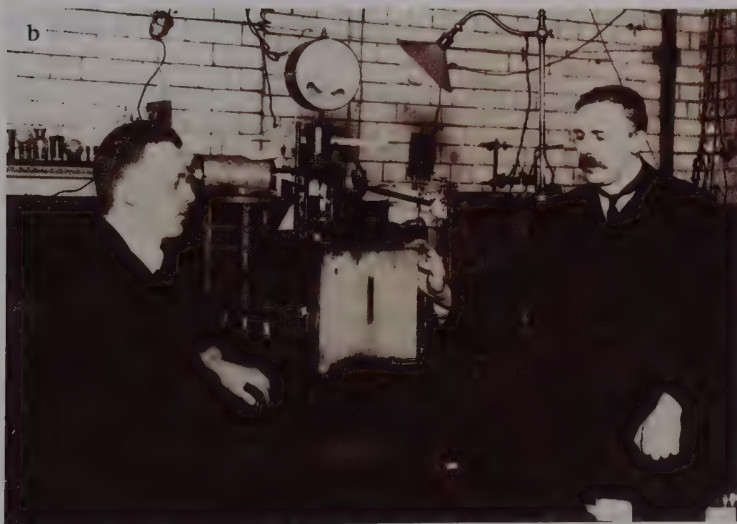
● Figure 1.7 Geiger and Marsden's experiment, which investigated how \alpha -particles are deflected by thin metal foils. a A drawing showing the arrangement of the apparatus. b Ernest Rutherford (right) and Hans Geiger using their apparatus for detecting \alpha -particle deflections. Interpretation of the results led Rutherford to propose the nuclear model for atoms.
