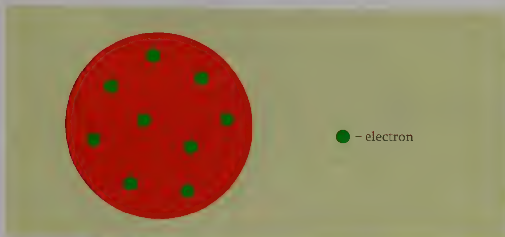
● Figure 1.6 J. J. Thomson's 'plum-pudding' model of the atom. The electrons (plums) are embedded in a sphere of uniform positive charge.
