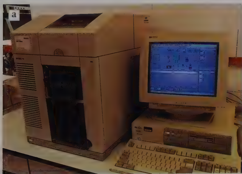
● Figure 7.16 a Capillary electrophoresis equipment. b Capillary electrophoresis enables the separation of organic molecules to take place under the influence of a high voltage. This electrophoretogram shows the retention times for compounds in a mixture; different compounds pass through the capillary tube at different rates. As each compound emerges from the capillary tube, its ultraviolet spectrum is also recorded. The vertical axis shows the absorption of ultraviolet radiation for each compound at certain wavelengths.
