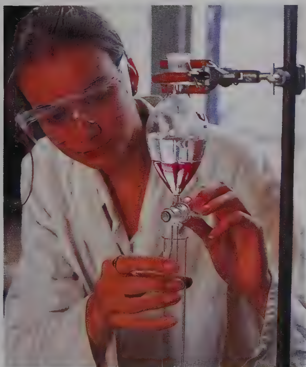
● Figure 7.13 A separating funnel enables the pink organic layer to be separated from the aqueous layer.
