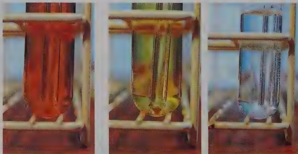
● Figure 10.5 The reaction of ethene with a solution of bromine. This characteristic reaction provides a test for an alkene (table 10.1).
