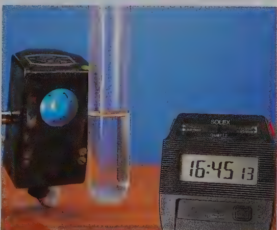
● Figure 9.4 The reaction of bromine with hexane in ultraviolet light.
