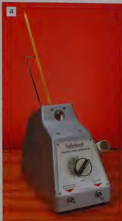
● Figure 7.15 a A simple apparatus used to determine melting point. b Close-up of crystals melting in the apparatus. c Diagram of a Thiele tube apparatus, also used to determine melting point.
