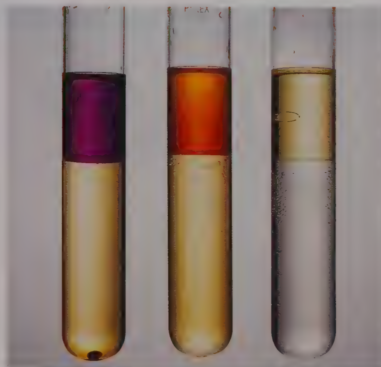
● Figure 6.3 Colours of halogens in cyclohexane (upper layer) and water (lower layer).
