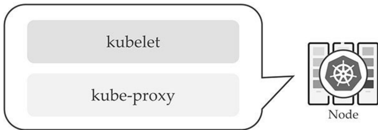
Figure 9.3: Node components in Kubernetes
