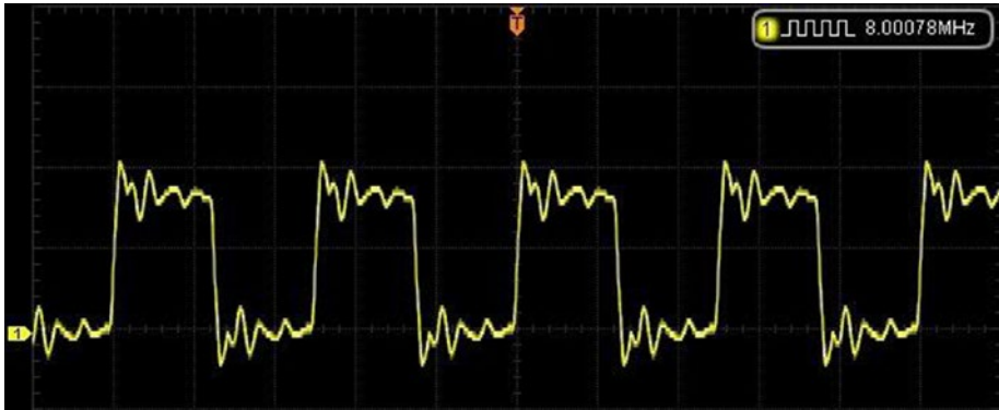
Figure 15-5. The HSE MCO trace (note how similar this is to Figure 15-4)
