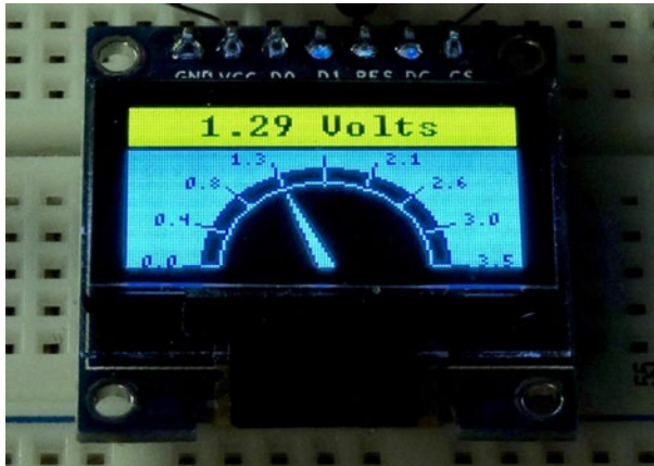
Figure 12-5. The demonstration program produces a voltmeter graphic on the OLED
