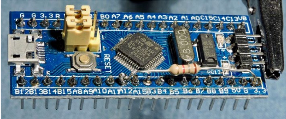
Figure 7-1. Correcting the USB pullup by addition of a 1.8-kohm resistor
