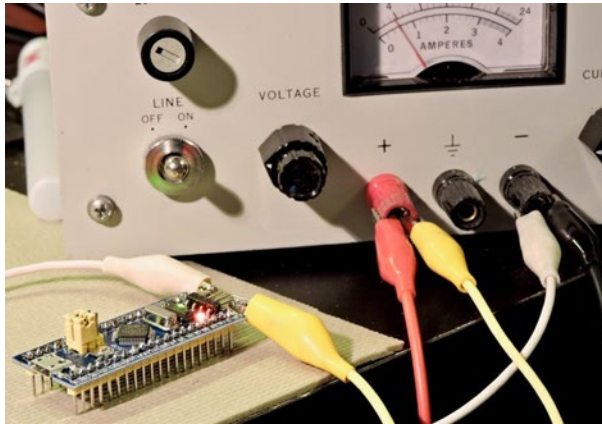
Figure 3-5. The STM32F108C8T6 blinking and powered by an HP 6284A power supply using the top header strip (+3.3 volts)
