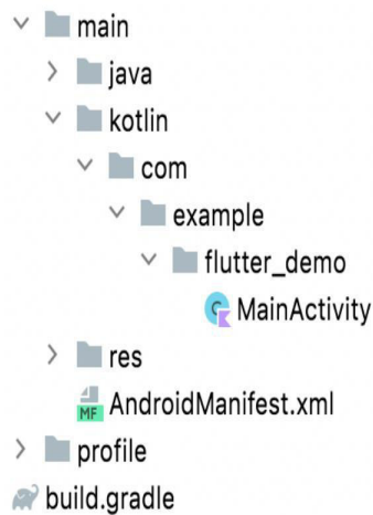
Figure 9.2: Default Android native project structure
