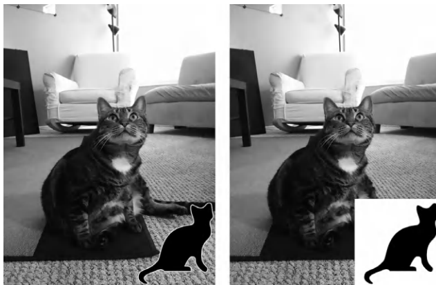
Figure 21-13: The program resized zophie.png and added the logo (left). If you forget the third argument, the transparent pixels in the logo will appear as solid white pixels (right).
