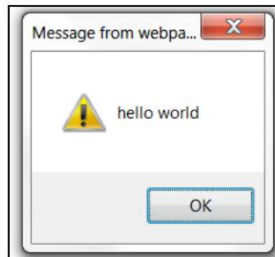
Alert message for the mnnsss variable after the script opened in Internet Explorer
