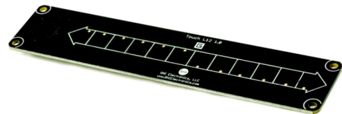
Figure 13-6 Multiple capacitive touch pads arrayed as a strip, made by GHI Electronics.
