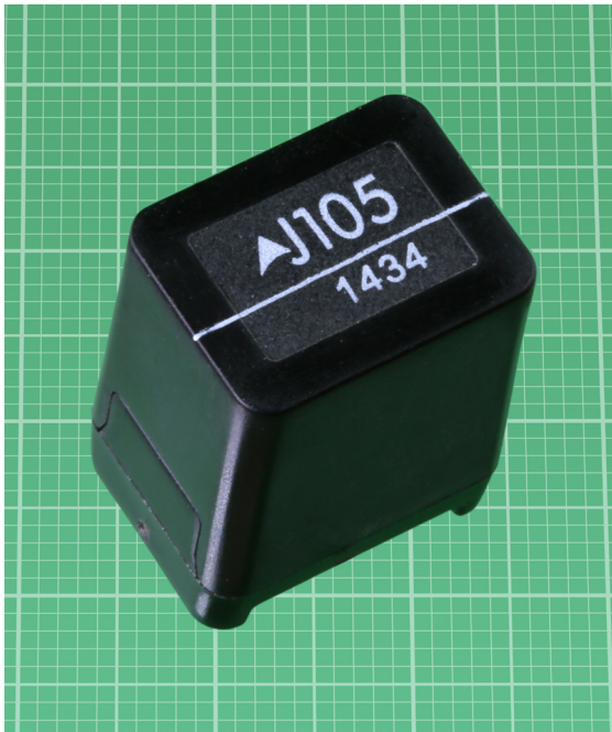
Figure 24-7 This inrush current-limiting PTC thermistor by TDK is packaged in a flame-retardant case. The background grid is in millimeters.
