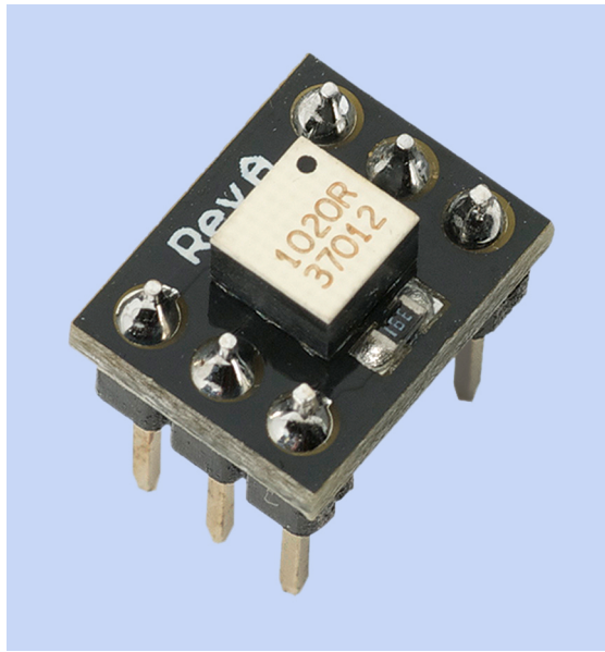
Figure 8-9 A 2-axis tilt sensor mounted on a breakout board available from Parallax.
