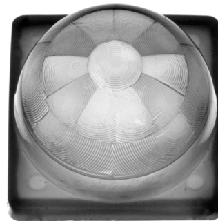
Figure 4-9 A mosaic weighted more toward sensing lateral motion. The grooves of the fresnel lenses are visible.
