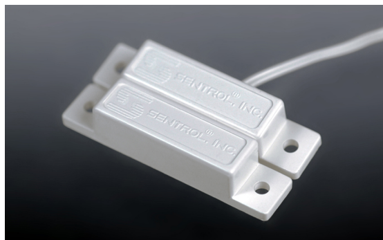
Figure 3-12 A typical alarm sensor to detect the opening of a door or window. The nearer module contains a magnet, while the module behind it contains a reed switch.
