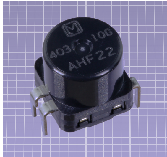
Figure 8-8 Exterior view of the Panasonic AHF22 tilt sensor. The background grid is in millimeters.
