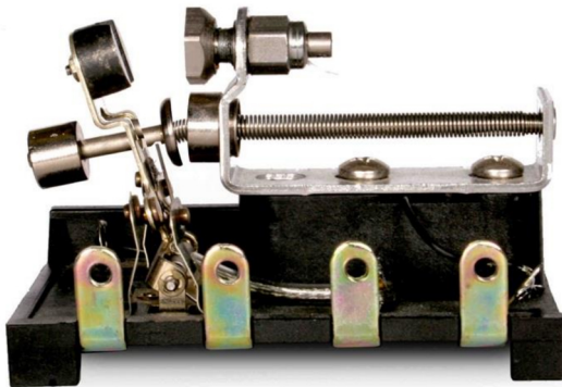
Figure 11-6 A magnetic vibration switch. See text for details.
