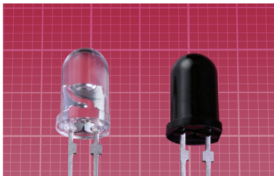
Figure 22-4 Osram infrared phototransistors SFH300 (left) and SFH300FA (right). The background grid is in millimeters.
